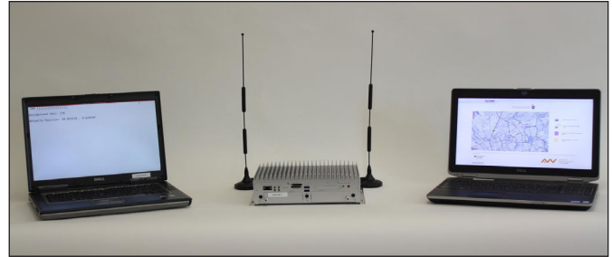
Figure 5: Demo Setup: Simulation of a Ko-HAF vehicle (left), communication box and a browser based visualization of the vehicle to server communication
